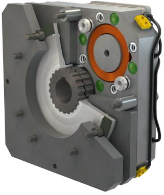
Left: The ROBA quatrostop brake systems have four individually switchable and inspectable braking circuits, functioning without doubling the braking torque in an emergency stop
