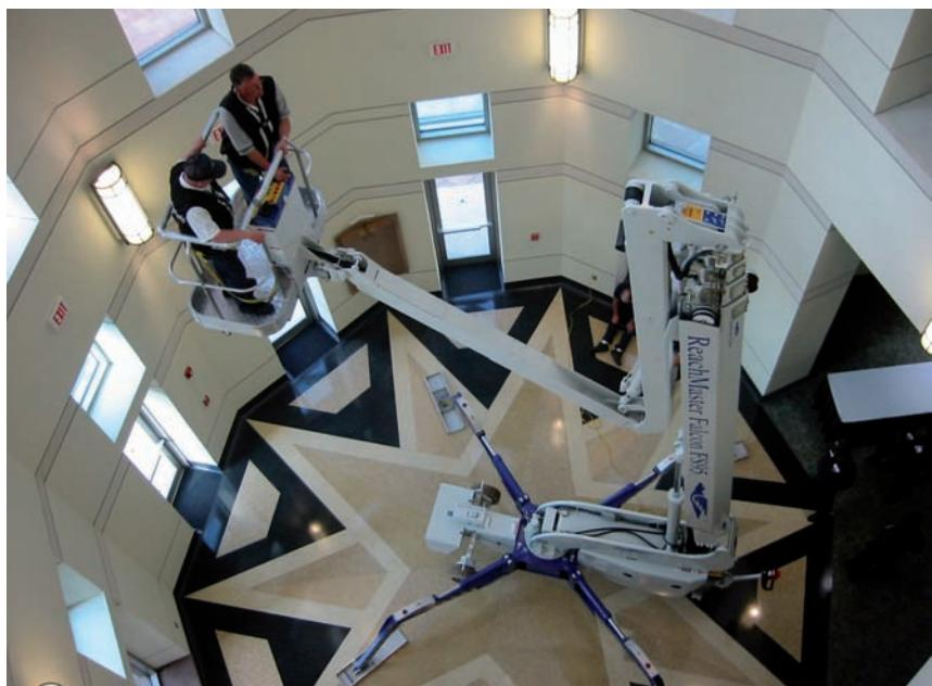
**Above:** There was less than 0.5in to clear the wall when erecting the main boom in the 20ft-wide rotunda
